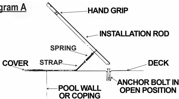
Place heel of rod behind raised anchor. Slip spring over anchor by moving handle away from the pool wall. Step down on spring. Remove installation rod by rotating 180 degrees and cover is then installed. (Diagram B)
