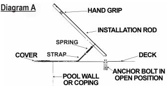
Place heel of rod behind raised anchor. Slip spring over anchor by moving handle away from the pool wall. Step down on spring. Remove installation rod by rotating 180 degrees and cover is then installed. (Diagram B)
