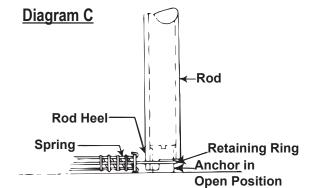
Next, press down and rotate 180 degrees. Heel of rod will force spring free of anchor. Tilt rod to release spring (Diagram D)
