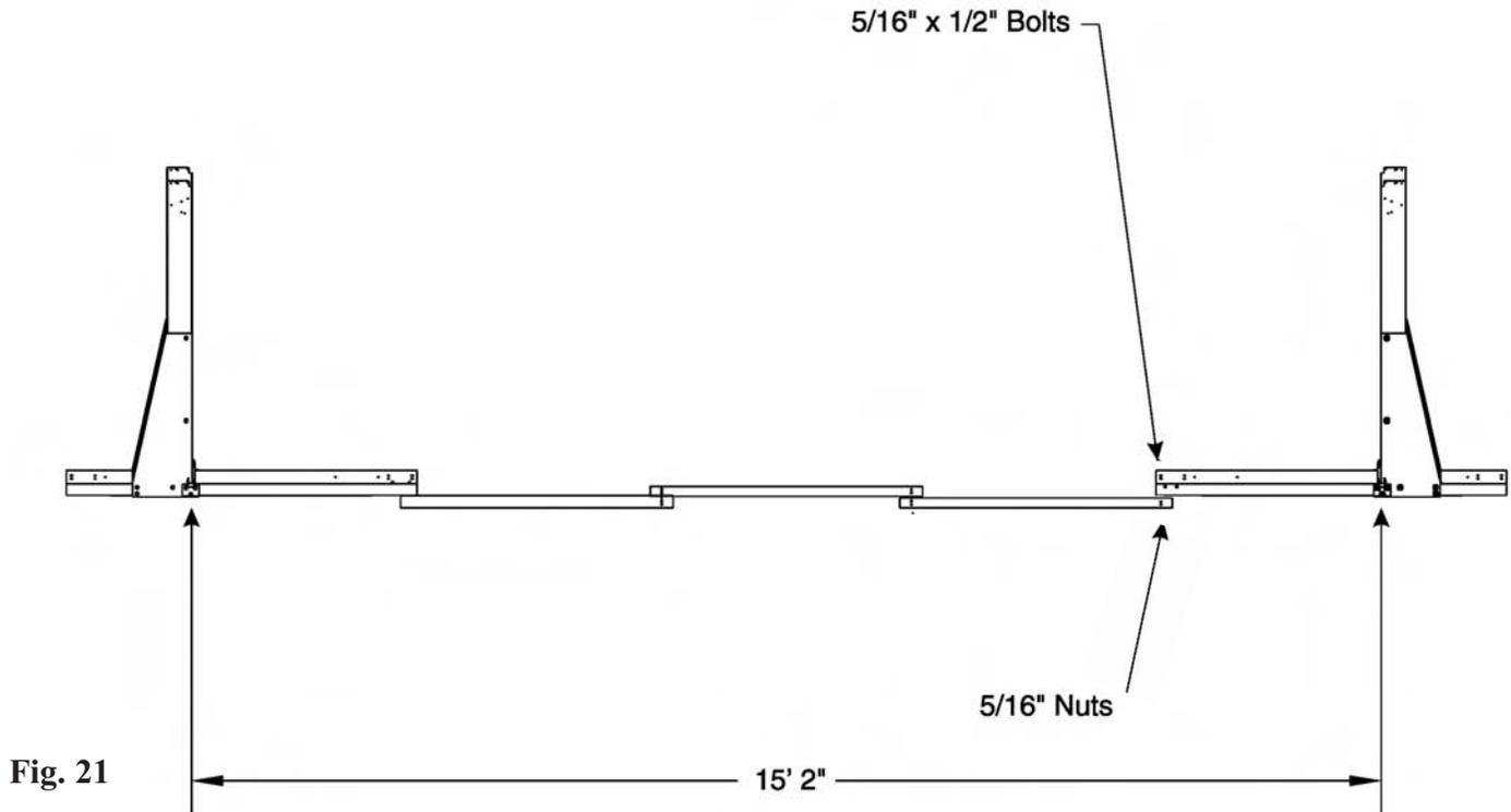
As you are bolting the strap to the strap end channels, add the end channel caps to the underside of the straps at each end as shown in Fig.22 and Fig.23.
