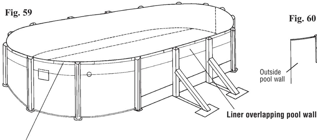
**Plastic coping installed at this time to hold liner in place**
