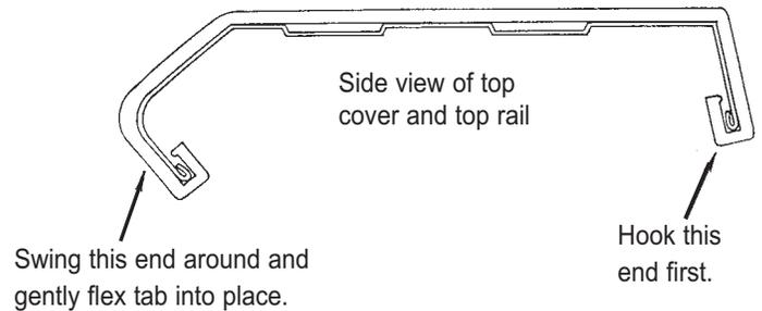
Bullnose rail is used for the illustration, but installation is the same for all 1 pc. clip-on resin covers.
