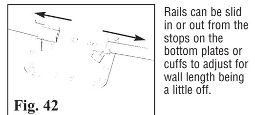
Rails can be slid in or out from the stops on the bottom plates or cuffs to adjust for wall length being a little off.
