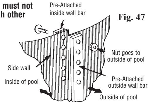
• If you are missing any hardware, do not leave empty holes in the wall joint assembly. Doing so will cause your pool to break! See your pool dealer for additional hardware in the case of a shortage.
