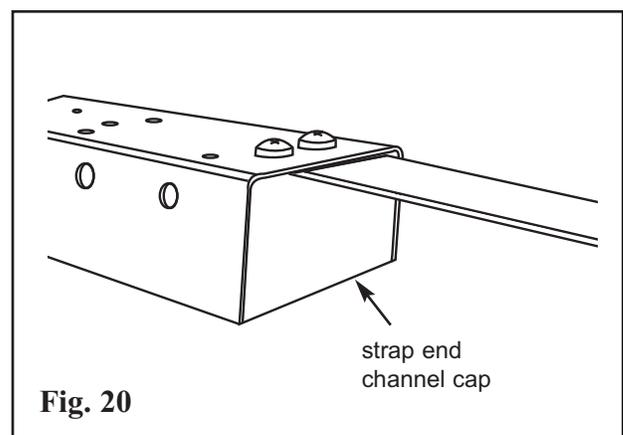
**ALTERNATE STEP 6 -ATTACHING STRAPS TO STRAP END CHANNELS FOR A BUTTRESS-FREE OVAL POOL ONLY:**
