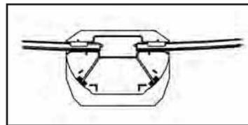
The bottom rail is inserted up to the dimple only.
