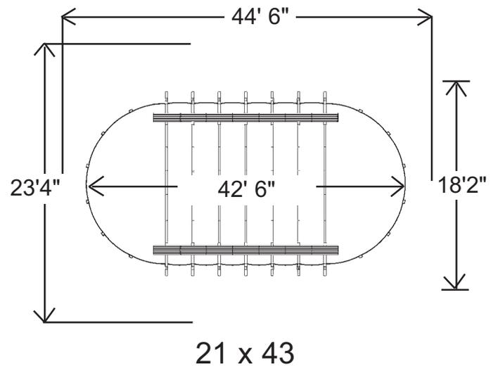
Note: All above diagrams are for Buttress-Free oval pools. If you have a traditional Buttress oval pool, you will need to add 3 feet to the width of the space needed for installation. The length measurement will not change.
