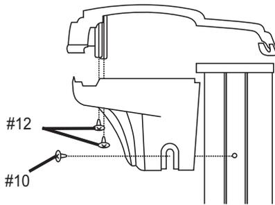
**2 PC RESIN TOP COVER:** Center small half over hole in the top plate as shown and attach with a #12 screw. Slide the large half over the small half and secure using two #10 screws.
