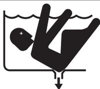
**SUCTION HAZARD. Can cause serious injury or death. Do not use this pump for wading pools, shallow pools or spas containing bottom drains, unless the pump is connected to at least two (2) functioning suction outlets.**
