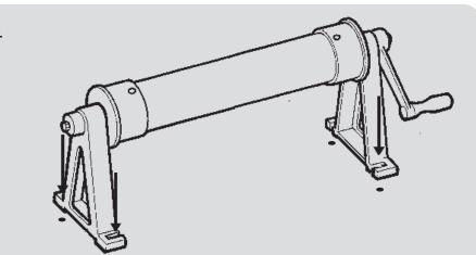
Using the two holes of the #4 A-frame (item #57) as guides, make two marks on deck for each #4 A-frame. With a 1/2'' concrete drill bit, drill a 1 1/2'' deep verticle hole at each mark.
