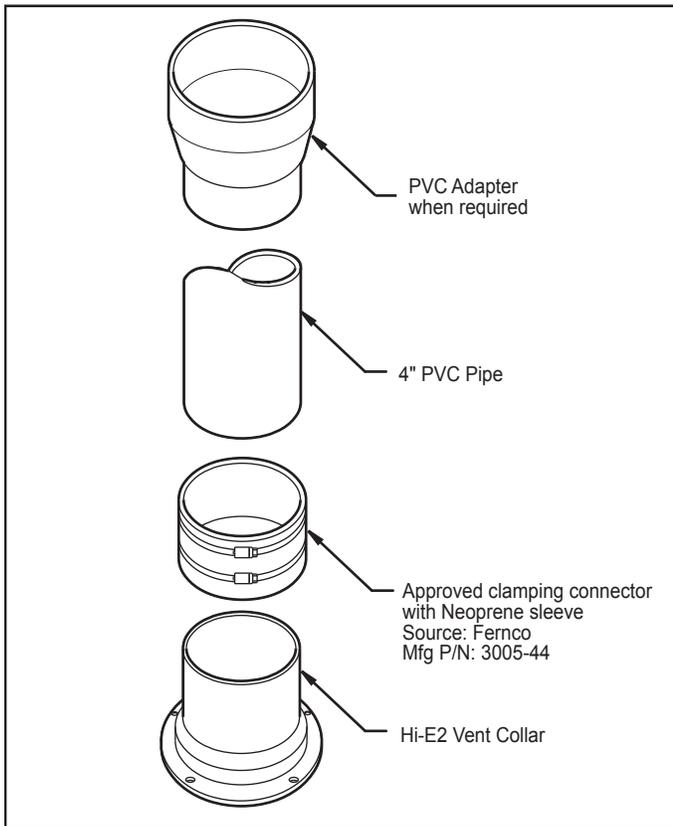
**Figure 7. Indoor vent connection, Hi-E2 pool heater.**
