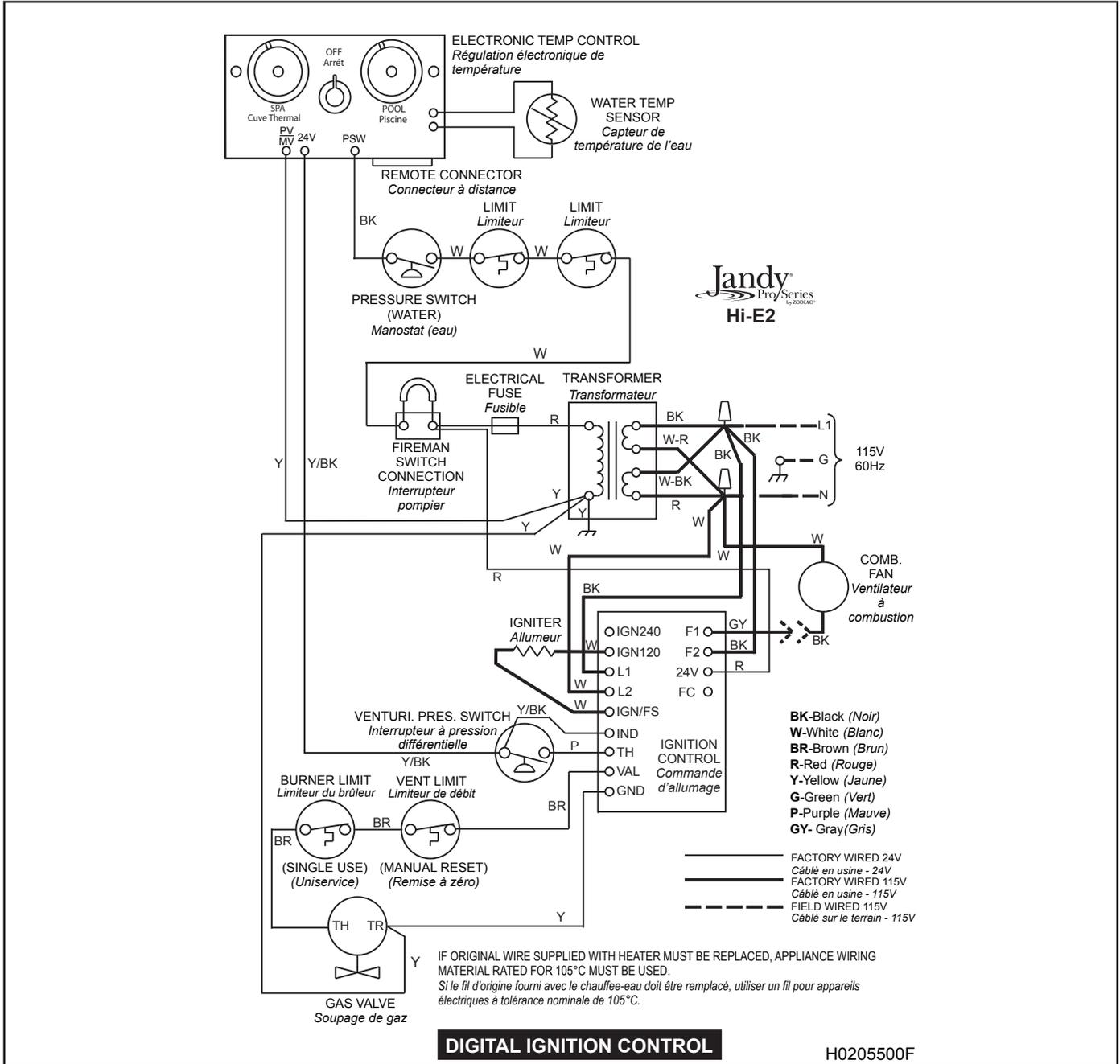
**Figure 15. Wiring diagram, Hi-E2 pool heater.**
