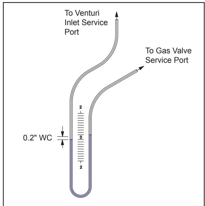
Figure 36. Gas pressure offset measurement with U-tube manometer.
