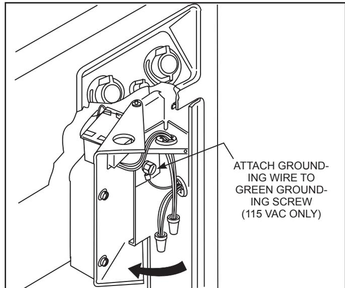
**Figure 14. Field wiring connections.**
