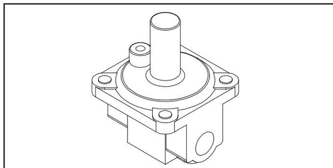
Figure 23. Step-down gas pressure regulator.
