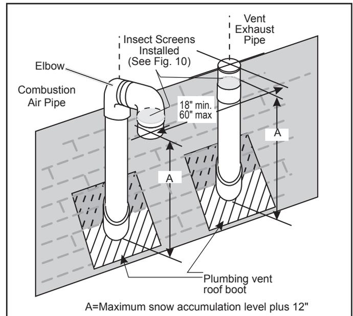
**Figure 9. Vent and combustion air terminals at roof.**
