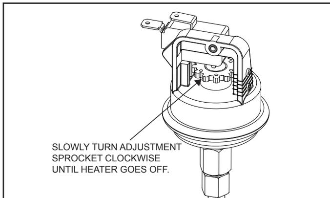
**Figure 24. Adjustment of pressure switch.**
