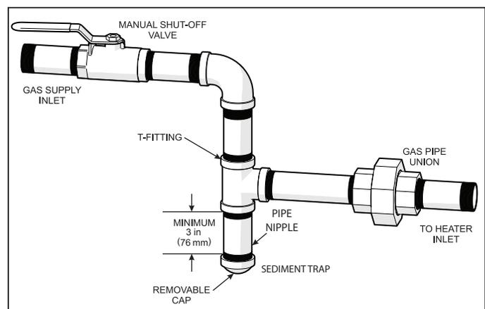
Figure 13. Manual Shut-off Valve and Sediment Trap.
