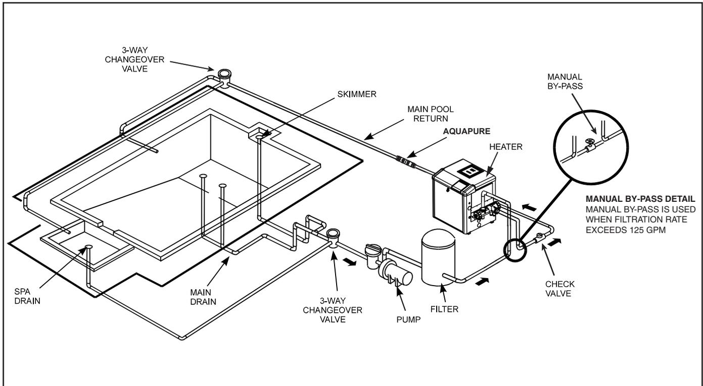
Figure 20. Typical water piping.
