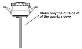
Carefully inspect the cleaned quartz sleeve for cracks. If any cracks in the quartz sleeve are found, the sleeve should be replaced. A broken quartz sleeve will allow water to enter the dry electrical chamber and attack the electrical components of the unit, which will cause them to fail and need to be replaced. Dispose of any broken glass in the proper waste receptacle. BROKEN QUARTZ SLEEVES, OR WATER DAMAGE CAUSED BY BROKEN QUARTZ SLEEVES, ARE NOT COV-ERED UNDER YOUR LIMITED WARRANTY.
