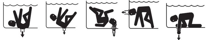
THIS PUMP PRODUCES HIGH LEVELS OF SUCTION AND CREATES A STRONG VACUUM AT THE MAIN DRAIN AT THE BOTTOM OF THE BODY OF WATER. THIS SUCTION IS SO STRONG THAT IT CAN TRAP ADULTS OR CHILDREN UNDER WATER IF THEY COME IN CLOSE PROXIMITY TO A DRAIN OR A LOOSE OR BROKEN DRAIN COVER OR GRATE.
