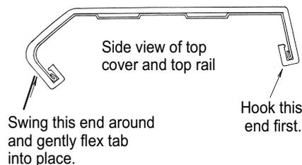
\*Bullnose rail is used for the illustration, but installation is the same for all 1 pc. clip-on resin covers.
