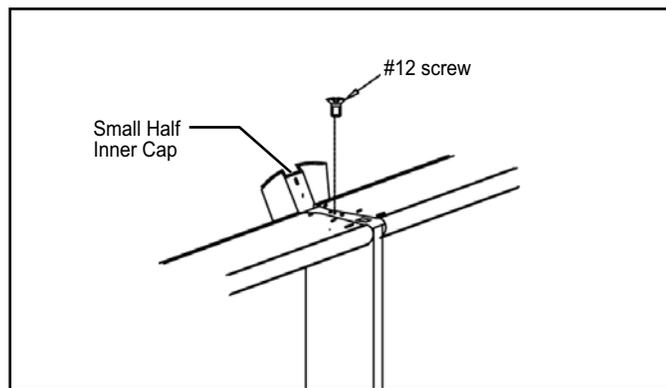
2) Attach the resin outer Top Cap using a #12 screw into hole. Put the grill over the screw when finished. See Diagram below.
