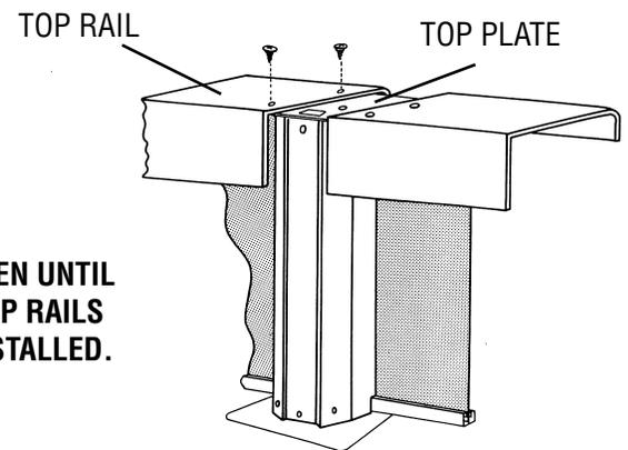
**\*USE TWO PEOPLE FOR INSTALLATION. IF A TOP RAIL FALLS INTO THE POOL, IT CAN CUT THE LINER.**
