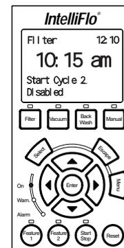
This screen shows the filter cycle as “Disabled” for a start/stop cycle (Cycles Per Day programmed to 1). These screens will still display even if they are not enabled.
