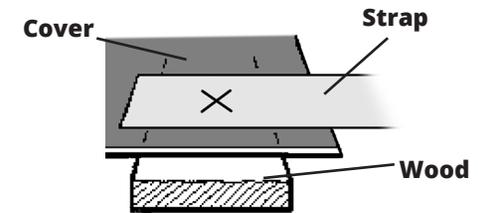
Position the blue strap on the cover. Cross cut through the strapping and the cover. Ensure that the hole in the strapping is at least 1" from the end of the strap and that the hole in the cover is at least 2" from the end of the cover. If possible fold the edge of the cover over so that you put the grommet through two layers of cover for extra reinforcement. This will ensure that the Grommet fits securely onto both the cover and the strap, and will help to prevent tearing.
