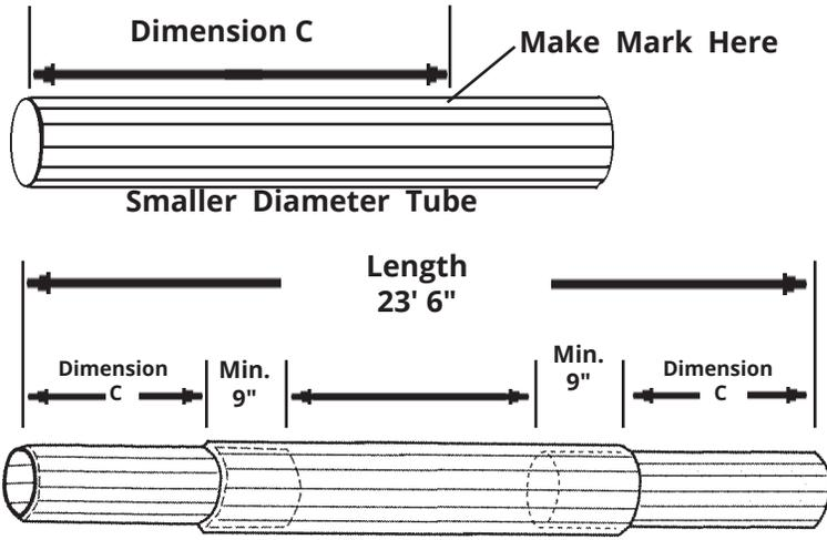
Insert smaller diameter tubes into the large diameter tube, up to the Dimension C mark, as shown. The total length of the tubes should be approximately equal to the corresponding value in Column B. See example on reverse.
