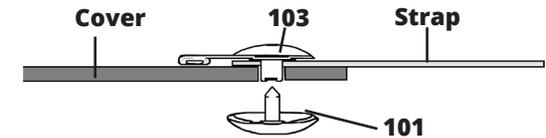
Insert the Female Grommet through your cut in the strapping and the cover. Ensure that the material is completely pushed down on the shaft. Insert the Male Grommet into Female Grommet. Once in place, hit with a hammer until secure. **(Caution - excessive force will break the grommets).**
