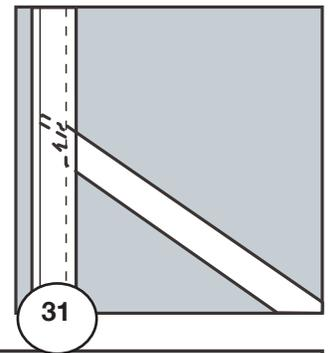
Very important: as you swing the diagonal down, make sure you apply constant upward pressure on the end of the diagonal brace with the tabs to ensure they stay fully locked in position in the slots.
