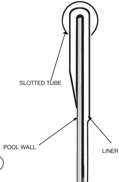
NOTE: Some liners may fit very tightly, it is better to install uprights, top plate and rail before going onto next step. See Section 4.
