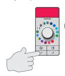
Push and hold the RESYNC button for 3 seconds
