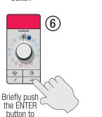
The Light Controller will indicate that a new countdown timer has been set by blinking LED 5 (see LED Indicator Codes) and then revert to Show/Color mode.
