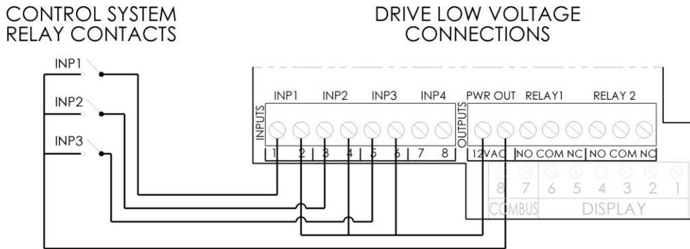
**Note:** For third party controls and Hayward controls that are not software compatible. Connection wire must be rated for a minimum of 300V. See section 5.6.11 for more details.
