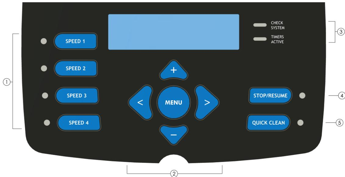
1. **Preset Speeds:** Buttons labeled SPEED 1 thru SPEED 4 can be used to run the pump at a predetermined speed for a certain length of time. Preset Speed settings can be quickly updated using the + and - arrow buttons and then holding the desired speed button down for at least 3 seconds. When a speed is selected, the LED beside the button will illuminate to indicate operation.
