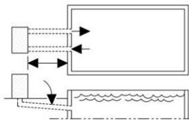
Locate pump as close to pool as practical and run suction lines as direct as possible to reduce friction loss. Suction lines should have continuous slope upward from lowest point in line. Joints must be tight (but not over-tightened). Suction line diameter must equal or be larger than the discharge line diameter.
