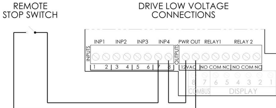
**Note:** Connection wire must be rated for a minimum of 300V. Switch must be latching type; pump is stopped when circuit is closed.
