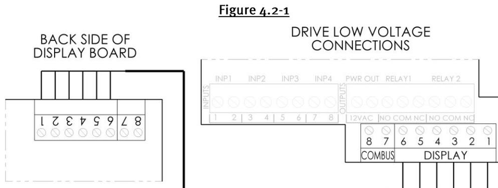
**Note:** Connection wire must be rated for a minimum of 300V. Wire used may be up to 500 feet in length.
