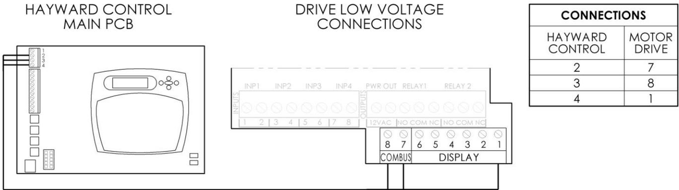
**Note:** For software compatible Hayward controls only (minimum software revision requirements: Pro Logic/Pro Plus 3.00, OnCommand 1.00, ECommand 2.65, ECommand 4 2.80, and Aqua Logic/Aqua Plus 2.65). Connection wire must be rated for a minimum of 300V. Wire used may be up to 500 feet in length.
