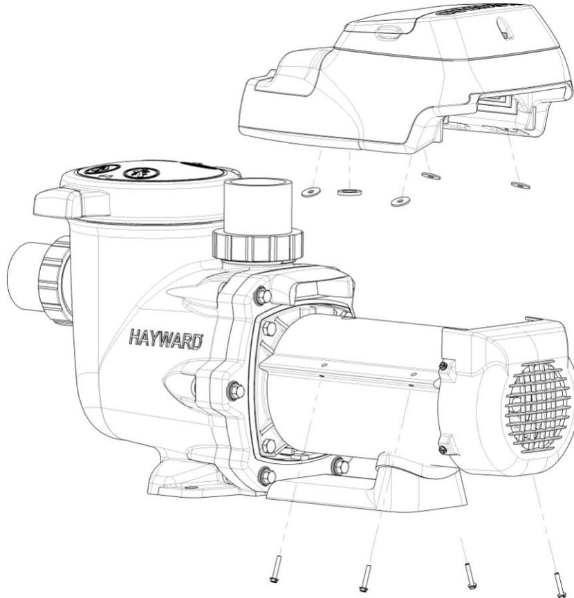
**Note:** Motor leads must be disconnected prior to removing drive, and reconnected when new drive is mounted. Take care to ensure that the motor leads are not pinched between the drive enclosure and the motor during assembly. The drive mounting screws must be tightened to 30 inch-pounds.
