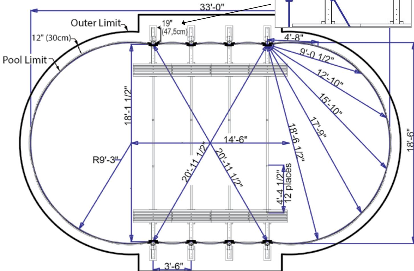
Perimeter 1047" (hole to hole)-Track length measured in track slot
