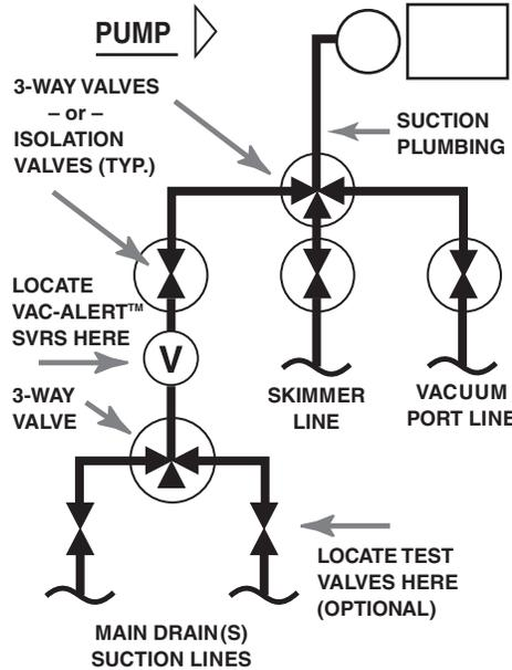
A: Always Locate The Vac-Alert™ SVRS On The Main Drain Suction Line. SVRS Unit Must Be Mounted In The Vertical Position.
