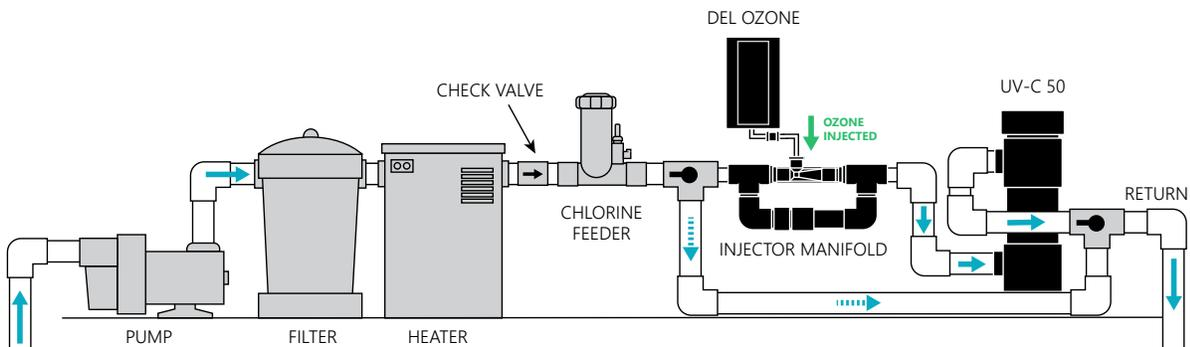
UV-C 50 WITH BYPASS VALVE & OZONE GENERATOR
