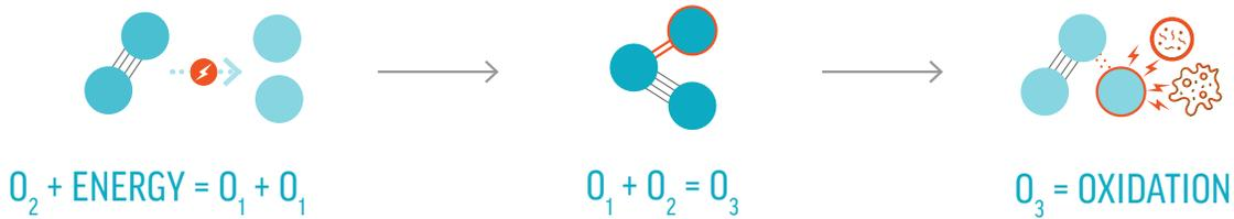
Energy created in the patented APG cell splits molecular oxygen (O<sub>2</sub>) into atomic oxygen (O<sub>1</sub>)
