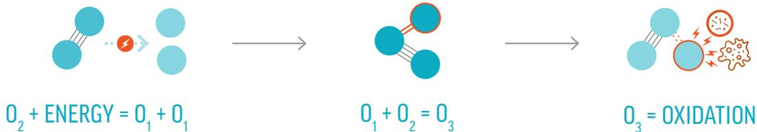
Energy created in the patented APG cell splits molecular oxygen ( $O_2$ ) into atomic oxygen ( $O_1$ )
