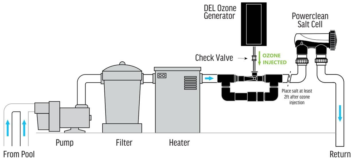
OZONE 25/50/100 WITH SALT SYSTEM & INJECTOR MANIFOLD KIT,
