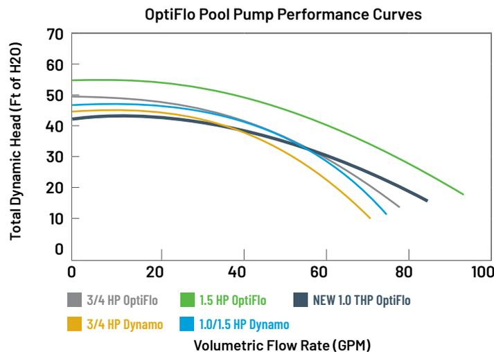
Note: The 3/4 HP OptiFlo, 1.5 HP OptiFlo and all Dynamo pumps represented here are non-compliant products included strictly for comparison. The new 1.0 THP OptiFlo represents the only series of pumps available for order.
