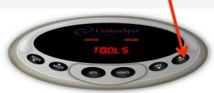
Step 3 - Press the Mode up or Mode down buttons to scroll through the submenus until you see one of the following submenus: Heat, Heat\*, Auto, Auto\*, or Chill
