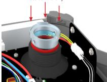
Gently lower the quartz tube into the unit until the Oring makes contact with the top of the black threaded sealing sleeve. Then place the aluminum compression washer and gasket on the quartz tube. Press down on the aluminum compression washer with an even steady pressure. Lift aluminum washer and check to make sure it is seated evenly around the circumference of the quartz tube. Replace aluminum washer.
