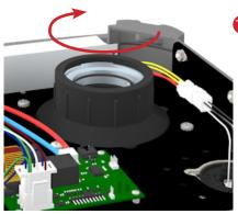
Screw on the quartz sealing nut to hand tight plus ½ turn. Turn pump on to check for leaks.
