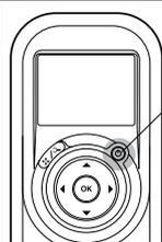
1. Press the On/Off button once. The remote control will start in manual direction control mode.
