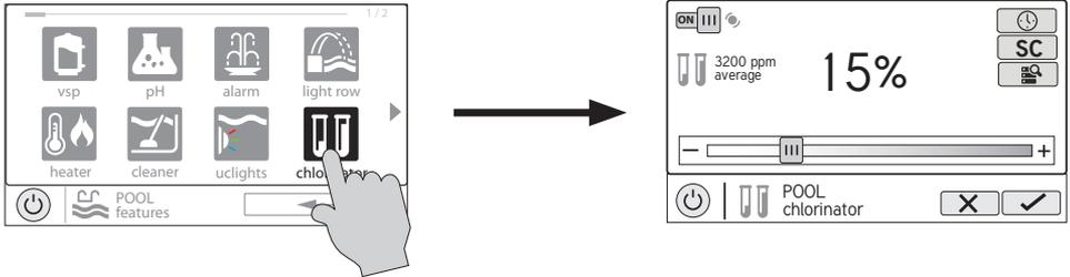
**Enable / Disable** - Slide this switch to enable and disable the chlorinator and then touch the Save button.
