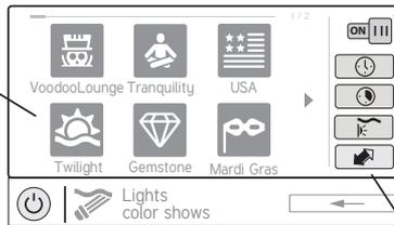
**Turn On / Turn Off** - Slide this switch to manually turn on/off the ColorLogic lights. This will override schedules or timer settings.
