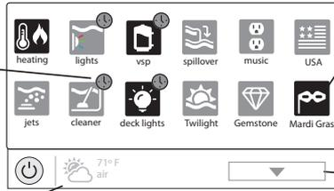
**Status** - Items that are highlighted are active or "On". In this example, the VSP pump, heater, deck lights and Mardi Gras light show are all On. Touching buttons in Simple Mode will turn the items On or Off.
