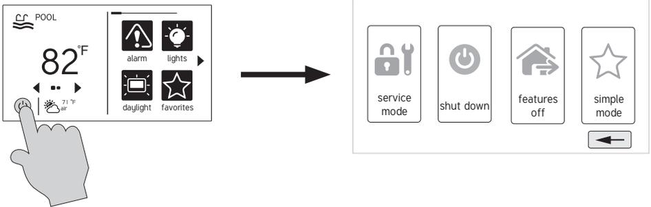
**Shut Down** - When Shut Down is selected, the OmniPL will turn off all pool equipment and report when it is safe to remove power. When this message is displayed, you can either power off the unit or restart the OmniPL by touching the large power button displayed on the left side of the screen.
