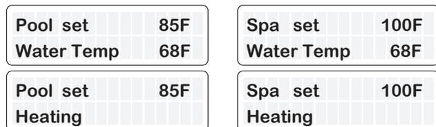
Figure 11. Modes POOL HEAT (CHAUFFAGE PISCINE) et SPA
