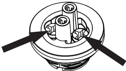
USE A MANUAL PHILLIPS HEAD SCREWDRIVER TO ENSURE THAT THE 2 SCREWS INDICATED ARE FULLY SEATED. PROCEED TO STEP 8.
