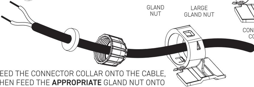
FEED THE CONNECTOR COLLAR ONTO THE CABLE, THEN FEED THE **APPROPRIATE** GLAND NUT ONTO THE CABLE
