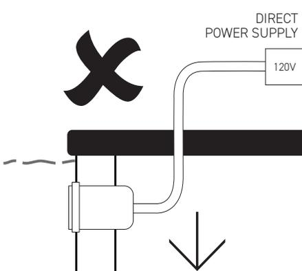
**1B:** A 12V AC TRANSFORMER **MUST** BE INSTALLED BETWEEN THE 120V POWER SUPPLY AND POOL LIGHT
