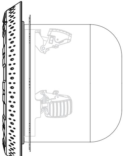
TIGHTEN THE THREE CAM LOCK SCREWS EQUALLY AND IN ROTATION, AS SHOWN, BY HAND UNTIL YOU FEEL THE NICHE ADAPTOR IS SECURE IN PLACE
