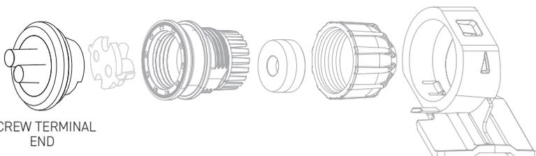
CHECK IF SCREWS ARE PRESENT IN THE TOP OF THE SCREW TERMINAL END
