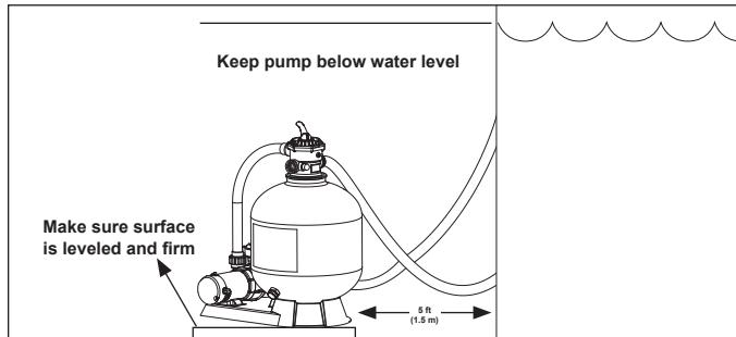
Although the pump is designed for outdoor use it is recommended that the installation consider the following:
