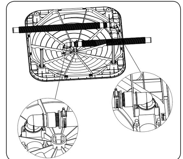
NOTE: The short hose is only used to connect multiple solar heaters together.
