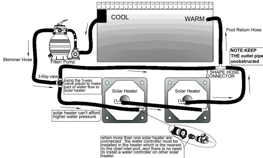
NOTE: The connections here show the water flowing into the Solar Heater through the center connector and out through the side hose connector. This diagram is for reference only as the flow may be reversed if you choose (i.e. the water flow coming in through the side hose connector and out through the center hose connector). The WATER CONTROLLER must put into the water inlet position.
