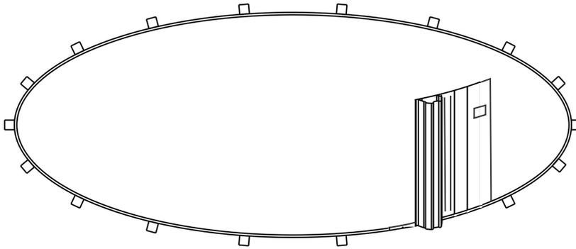
**Throughout installation, be sure to verify that the Bottom Rail distance from center is consistent.**
