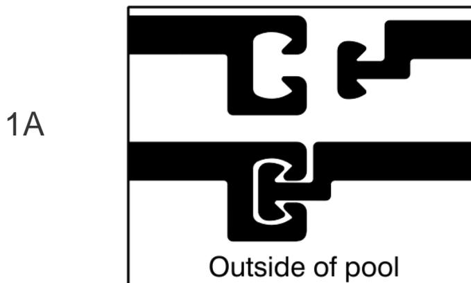
You may need to gently tap the slat down using a rubber mallet or hammer using a block of wood to prevent any denting or nicking of the slat. The last slat installed is often particularly tricky. The use of 3-in-1 household oil or WD-40 often helps (do not use motor oil).
