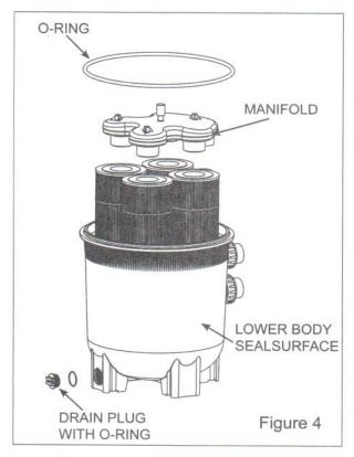
By recording the initial starting pressure (with clean filter elements) a determination can be made when the filter cartridge elements should be replaced rather than cleaned. After the filter elements have been cleaned and reinstalled if the starting pressure is higher than 6 PSI above the starting pressure with the new filter cartridge elements, the filter cartridge elements should be replaced the next time the gauge arrow reaches the red arrow.
