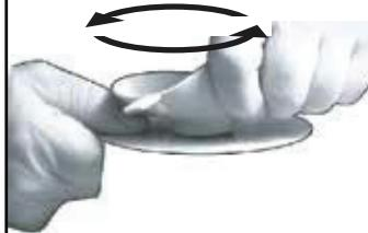
**A3)** Twist the Step Cup to ensure that the mushroom ring has entirely cleared the wall thickness. If it has, the suction cup should rotate freely.
