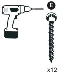
1) Affix the deck supports to the deck with the screws supplied.
