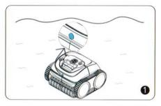
About 20 seconds of auto calibration on the floor, the indicator light will turn flashing blue. The cleaner is ready to clean.
