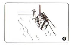
You can insert the included hook into a pool rod and lift the cleaner out of the pool.
