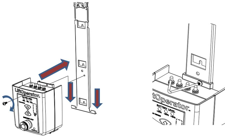
13. Remove the battery from the accessory carton and carefully attach to controller.
