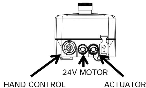
15. The 24V motor cable will be secured to the mast in **step 18**. For the moment, simply string it through the housing mast hole. Plug the 24V motor cable (red stripe) into connector #1 on the Control Box. Make sure the plug is secure and completely seated. Allow the 24V motor cable to hang freely and untangled from the first pre-installed clip.
