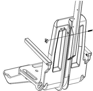
27. Attach foot rest to seat with bolts and thumbnuts.
