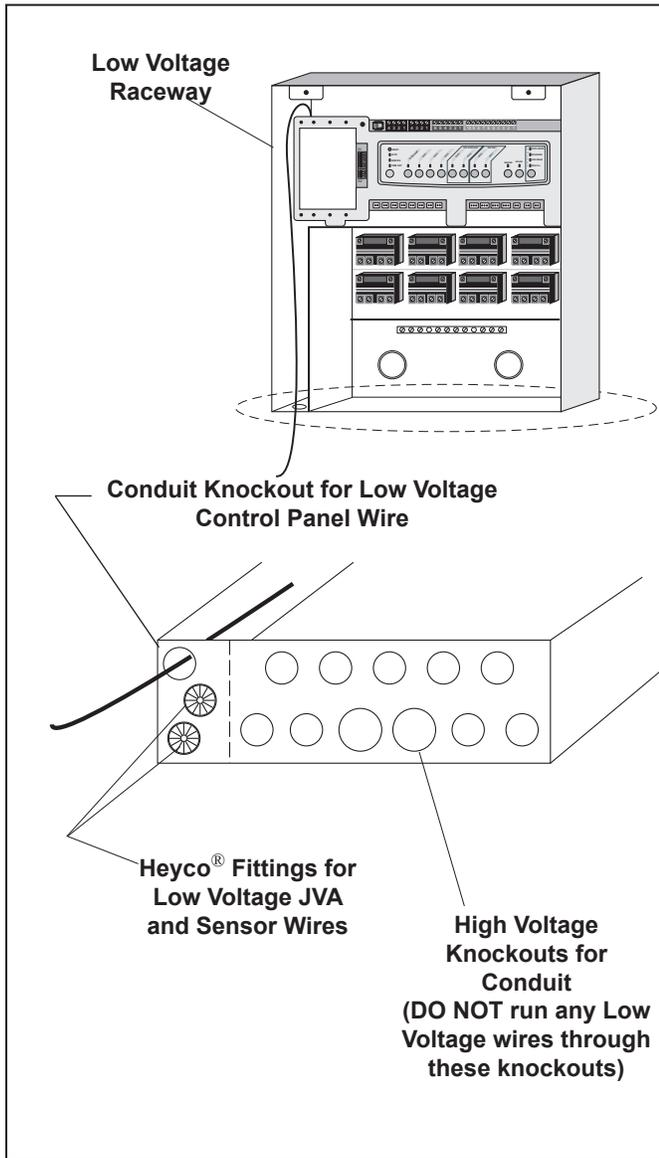
Figure 12. Control panel Cable to Power Center PCB
