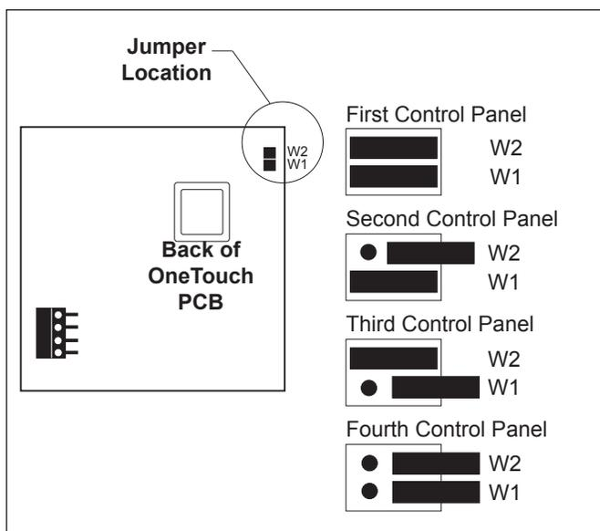
Figure 32. Jumper Settings for Multiple OneTouch™ Control Panels
