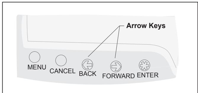
Figure 37. AquaLink® RS All Button Control Panel Buttons
