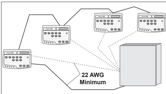
Figure 25. Installing Multiple All Button Control Panels
