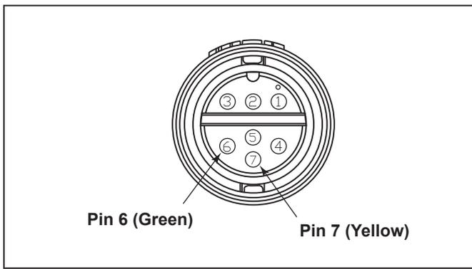
Figure 14. Cable Connector at the Pump Side
