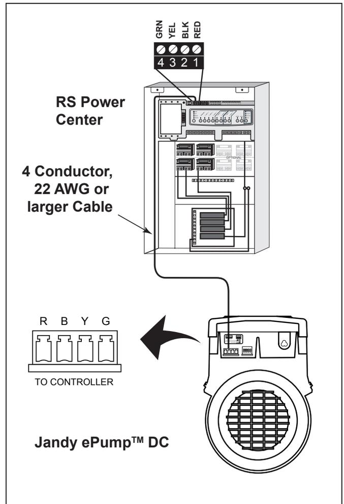
Figure 13. Low Voltage Wiring for Jandy ePump™ DC
