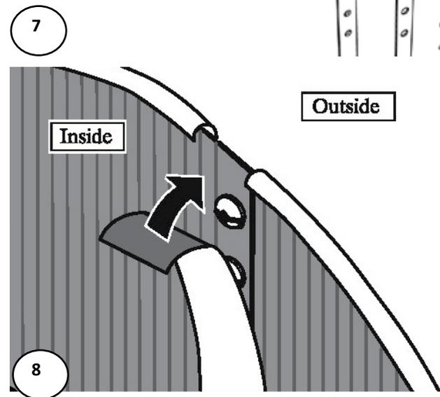
When tightening the screws start from either the top and go down or vice versa. Do not start a few screws from top and a few from the bottom to meet in the middle, this can cause problems later on.
