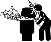
THIS FILTER OPERATES UNDER HIGH PRESSURE. WHEN ANY PART OF THE CIRCULATING SYSTEM (e.g., FILTER LID, PUMP, FILTER, VALVES, ETC.) IS SERVICED, AIR CAN ENTER THE SYSTEM AND BECOME PRESSURIZED. PRESSURIZED AIR CAN CAUSE THE LID TO SEPARATE FROM THE TANK BOTTOM WHICH CAN RESULT IN SEVERE INJURY, DEATH, OR PROPERTY DAMAGE. TO AVOID THIS POTENTIAL HAZARD, FOLLOW THESE INSTRUCTIONS.
