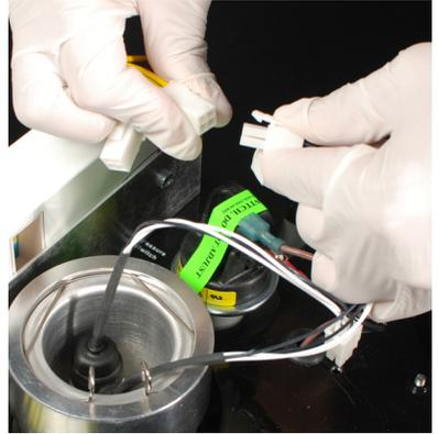
1. Turn off all power to the ULTRA UV2 unit and all other pool equipment. Unplug the unit from its power receptacle or turn OFF the circuit breaker that is the ULTRA UV2's power source. Before proceeding to step 2 allow at least 15 minutes for the lamp(s) in the unit to cool.
