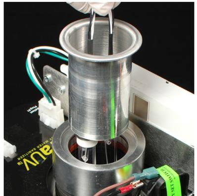
5. Carefully remove new lamp assembly from box. Insert lamp(s) into lamp holder. lamp(s) must be aligned and seated securely in the lamp holder. Roll the black o-ring(s) up onto the ceramic end of lamp from position A to B, Fig. 8. Gently insert lamps into the lower lamp retainer Fig. 9 and lower lamp assembly into unit.
