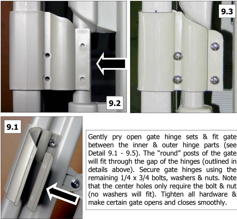
Gently pry open gate hinge sets & fit gate between the inner & outer hinge parts (see Detail 9.1 - 9.5). The "round" posts of the gate will fit through the gap of the hinges (outlined in details above). Secure gate hinges using the remaining 1/4 x 3/4 bolts, washers & nuts. Note that the center holes only require the bolt & nut (no washers will fit). Tighten all hardware & make certain gate opens and closes smoothly.
