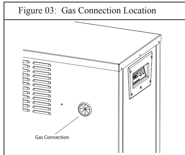
Reduction of gas supply pipe or tubing to the inlet of the heater gas valve must be made at the valve only and must match the valve inlet size (3/4" NPT).
