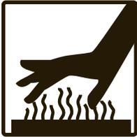
**⚠ WARNING: BURN HAZARD** The operation of the heater with the pump shut off could cause heater overheating and fire. Never operate heater with the pump shut off.
