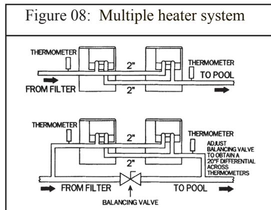
Figure 08 illustrates a multiple heater installation for very large pools with and without a manual bypass valve.
