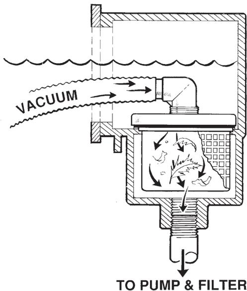
**MODEL SP11052** Furnished with 1-1/2" x 1-1/4" hose elbow. For use on Skimmer Model SP1090, front access style.
