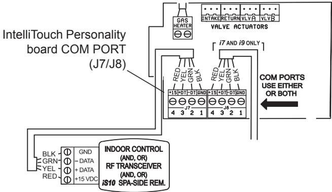
**Pin Configuration Pump to IntelliTouch control system pin configuration:**
