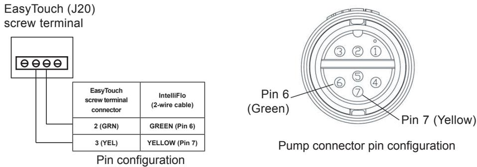
9. Insert the screw terminal onto the EasyTouch **COMPORT (J20)** board connector.
