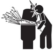
FILTER OPERATES UNDER HIGH PRESSURE. WHEN ANY PART OF THE CIRCULATING SYSTEM (e.g., LOCK RING, PUMP, FILTER, VALVES, ETC.) IS SERVICED, AIR CAN ENTER THE SYSTEM AND BECOME PRESSURIZED. PRESSURIZED AIR CAN CAUSE THE LID TO SEPARATE WHICH CAN RESULT IN SEVERE INJURY, DEATH, OR PROPERTY DAMAGE. TO AVOID THIS POTENTIAL HAZARD, FOLLOW THESE INSTRUCTIONS AND THE INSTRUCTIONS THAT CAME WITH AND THAT ARE ON THE FILTER.
