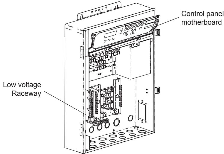
7. Strip back the cable conductors ¼ inch. Insert the two wires into the screw terminals on the board. Secure the wires with the screws.
