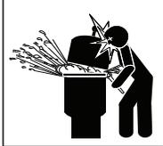
Install all electrical controls at equipment pad, such as on/off switches, timers, and control systems, etc. to allow the operation (startup, shutdown, or servicing) of any pump or filter so the user does not place any portion of his/her body over or near
