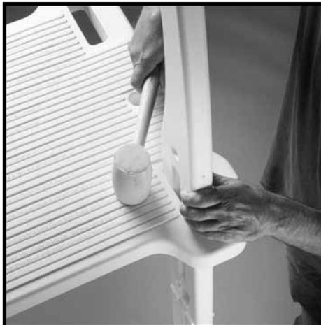
**#3:** Stand up the assembly and using a rubber mallet tap the Platform down until seated on the lugs on the Side Rails. IT MAY REQUIRE SEVERAL HARD BLOWS WITH A RUBBER Mallet TO SEAT THE PLATFORM ALL THE WAY DOWN ONTO LUGS.
