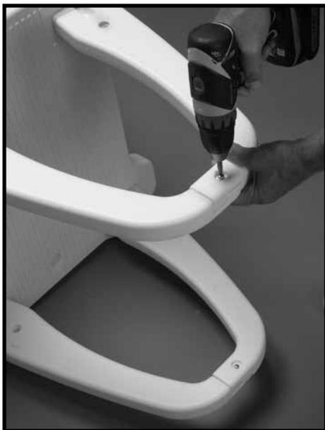
**#5:** Using two #10 x 3/4" self-tapping screws, connect the Handrails together by using one screw on the outside and one screw on the inside. Repeat for the remaining handrails.
