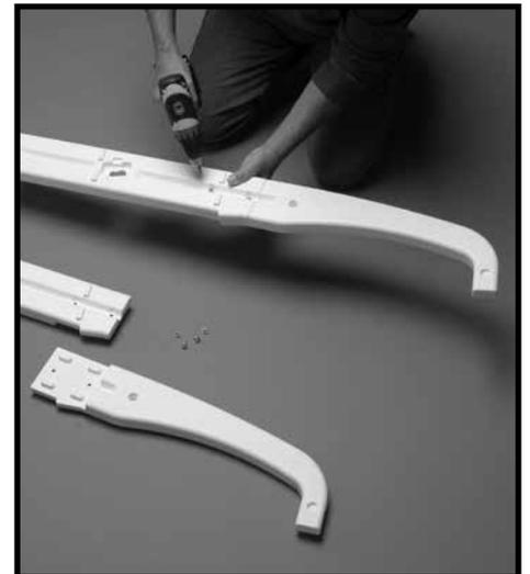
**#1:** Overlap the flat end of the Handrail onto the top of the Side Rail. Using two 1/4 - 20 x 5/8” bolts and two 1/4- 20 hex nuts, attach the Handrail to the Side Rail. Repeat for the remaining Side Rail.
