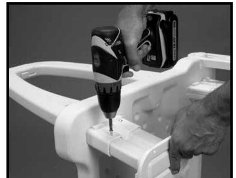
**#3:** Laying the ladder on its side, attach both Mounting Block assemblies to the ladder using two #10 x 3/4" self-tapping screws in each assembly.
