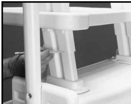
**#2:** Position the ladder so the Mounting Blocks sit flat. Using a pencil, mark the height on the Mounting Block Tubes. *NOTE: If necessary you may need to cut down the Mounting Block Rails with a hacksaw.*
