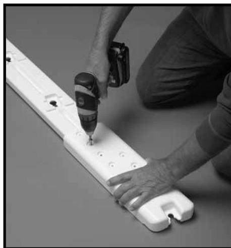
**#2:** Using two 1/4-20 x 1 1/2” long bolts and two 1/4-20 hex nuts, fasten the Adjustable Rail Boot to the Side Rail. Repeat for remaining Side Rail.
