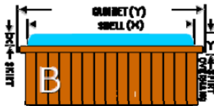
Figure 2. Measuring spa configuration with cabinet and wooden-edge trim
