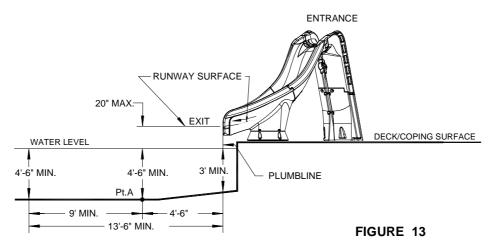
2. A minimum clearance area in front of the slide shall be maintained at all times as follows:
