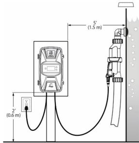
It is designed to be mounted on a vertical, flat surface, in a ventilated area.
