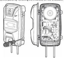
Locate the input power terminal block and loosen the 3 screws holding the factory installed power cord wires to the power terminal block.
