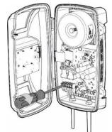
Position the wires on the input power terminal block. Tighten the three (3) screws and secure the wires correctly in place.
