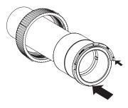
Snap retainer ring around the adapter.
