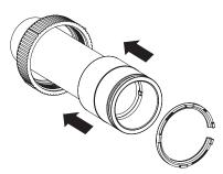
Slip the nut onto the fitting.
