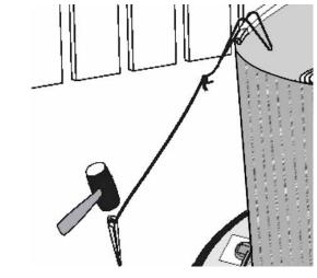
d. When uncoiling the wall, the skimmer and return holes are positioned toward the end of the wall. (Image 4)
