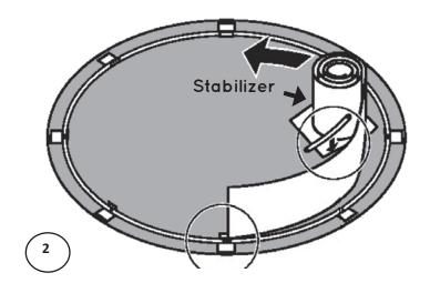
d. Set lengths of stabilizer onto the top edge of the wall as you uncoil it. (Image 2)
