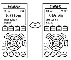
This example will run the pump for 24 hours. Start and Stop Cycle is displayed
