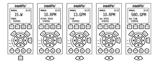
**Note:** No sensors except the flow control will work while in "Manual" mode. Suction Blockage will not work in this mode.
