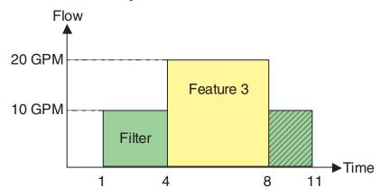
"Feature" 1 and 2 do not have time-of-day functions and do not affect the filter cycle time. The active time for "Feature" 1 and 2 will not be calculated into the reduced cycle time as shown in the above example.
