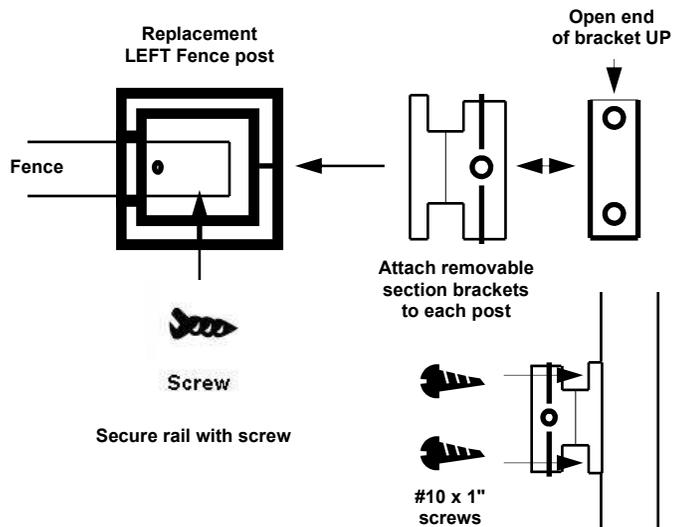
**Step 3** Remove the post hardware used to secure section in place (both sides of section). Keep this hardware & remember positioning as you will require it to reassemble. Remove fence section & remove the two line posts. Keep all hardware for reassembly. Note: you may have some extra hardware left over once complete as line posts have double for opposite sections. DO NOT REMOVE MOUNTING BRACKETS FROM POOL UPRIGHT POSTS
