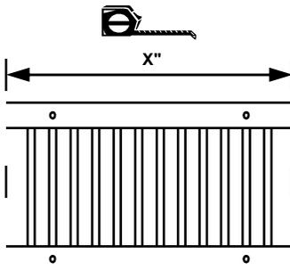
**Step 5** Measure distance from inside of bracket to inside of bracket from the left end post to the right end post. Mark this length/measurement on the fence section. Make certain to balance distance from each end picket on both ends of section so final installation looks neat & balanced. Cut rail ends accordingly
