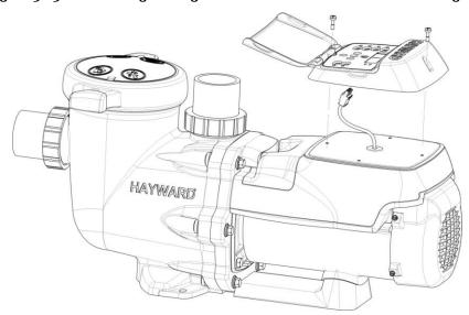
Figure 3.13-2: Adding the Blank Cover
