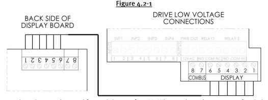
Note: Connection wire must be rated for a minimum of 300V. Wire used may be up to 500 feet in length.
