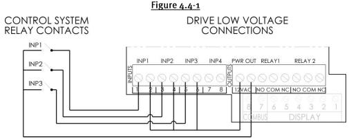
**Note:** For third party controls and Hayward controls that are not software compatible. Connection wire must be rated for a minimum of 300V. See section 5.6.11 for more details.
