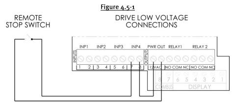
**Note:** Connection wire must be rated for a minimum of 300V. Switch must be latching type; pump is stopped when circuit is closed.
