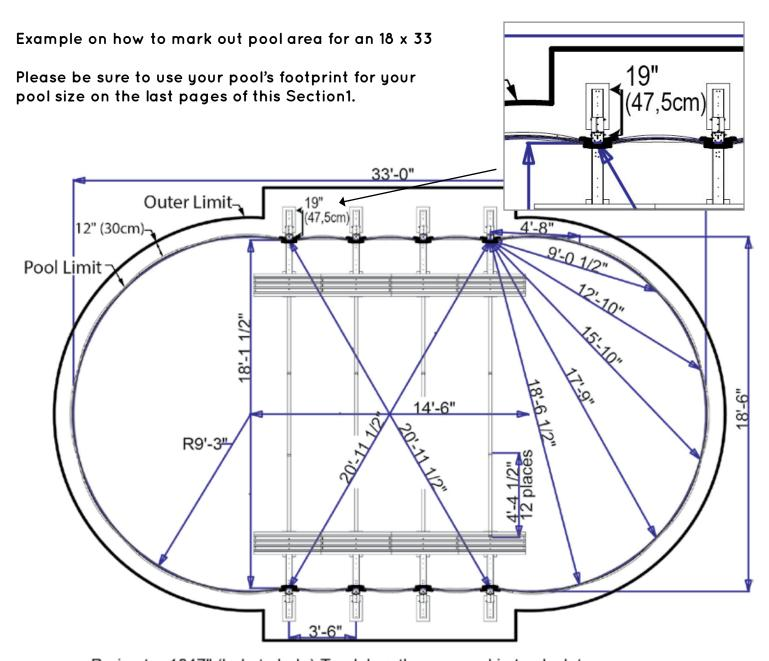
Perimeter 1047" (hole to hole)-Track length measured in track slot All dimensions are in inches
