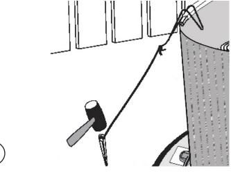
d. When uncoiling the wall, the skimmer and return holes are positioned toward the end of the wall. (Image 4)
